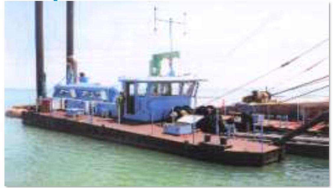
3 Dredgers CZ-400 Dredging depth 10 Meter 1130 HP
