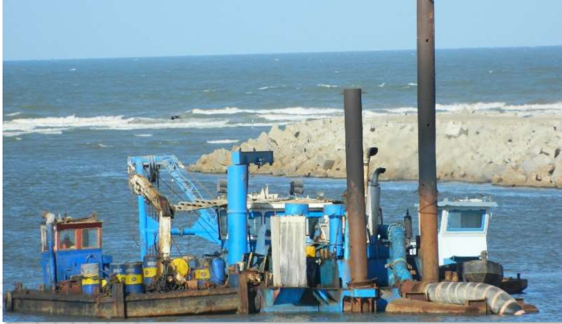
2 Dredgers CZ-500 Dredging depth 14 Meter 1742 HP
