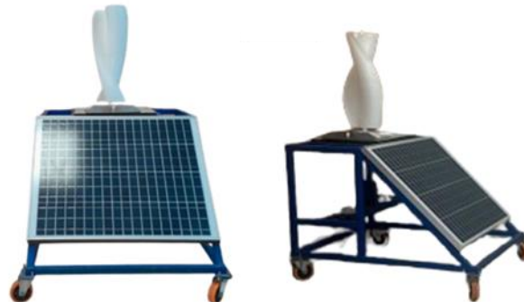
An isometric final view of the hybrid wind-solar unit prototype
