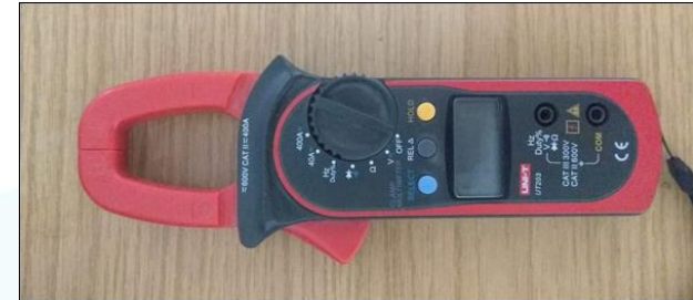
Multimeter device for the voltage and amperage measurements
