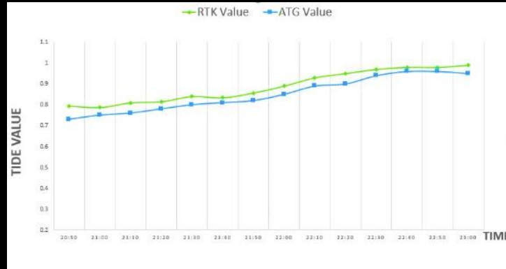
Comparison between RTK and tide gauge data distance about 1 km from the base station
