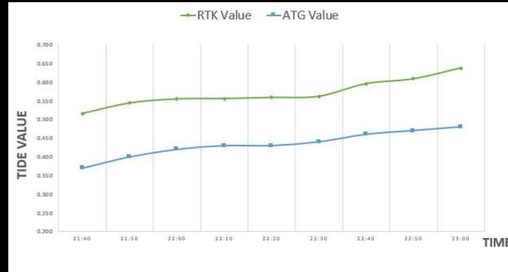
Comparison between RTK and tide gauge data distance about 10 km from the base station
